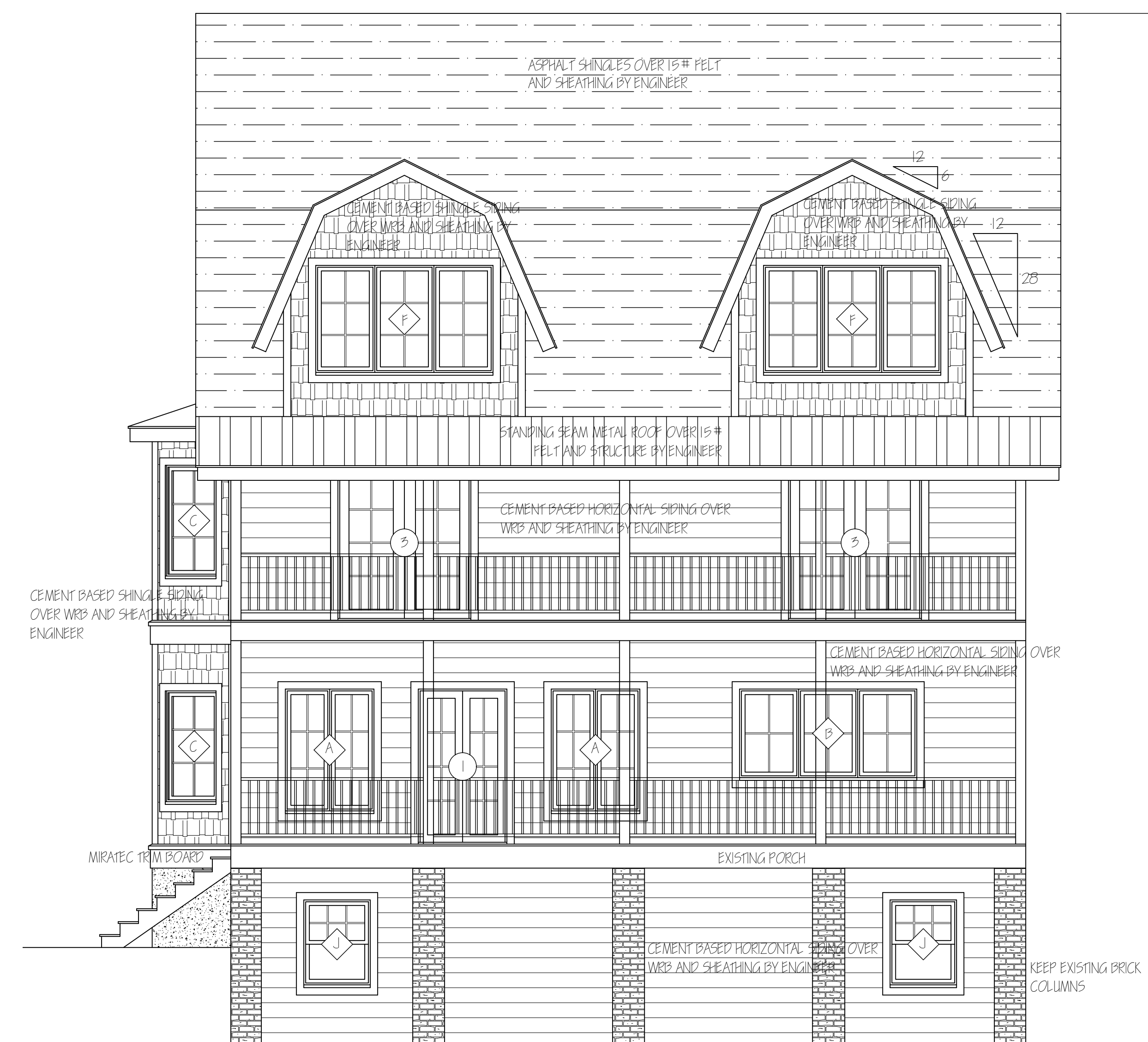
FRONT ELEVATION NORTH CAROLINA TERRACE VIEW
