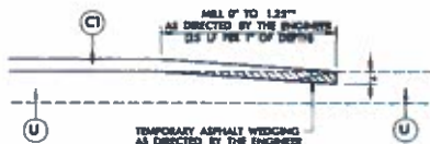
Detail Showing Method of Wedging
